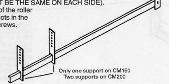
Slide on track support brackets and fasten to a suitable support square to the door and allowing the fall as above with 1 M8 x 40mm coachscrew. (Other supports will be fitted later). Fit rubber Buffers in rearmost track hole and adjust later to correct hole for door open position.
