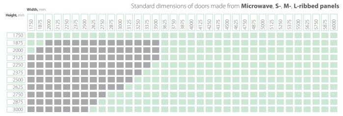
The chart shows the allowable size range. All doors are made to measure in 5mm increments in width and height.
