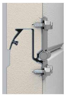
Self-tapping screws are positioned at the junction of the of external and internal sheets (4 layers of metal) which makes the fixing more durable. Reliable connection of steel sheets prevents panels from delamination in case of the door closing abruptly.
