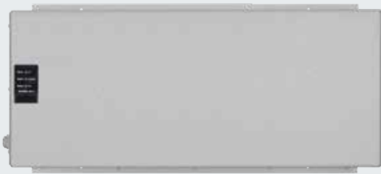
UPS system For bridging power failures of up to 4 hours, safety devices, warning lights, etc., remain functional, LED status display, automatic battery test, surge filter, dimensions: 560 x 235 x 260 mm (W x H x D), protection category: IP 20
