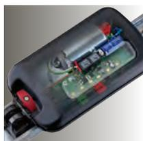
The motor control units' safety circuits monitor force levels many times every second. If the door encounters an obstruction, it is instantly sensed and the motor stops and reverses a short distance.
