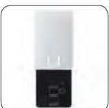
528 - 2 channel fingerprint scanner.
