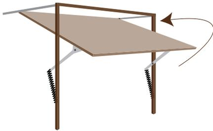
**Canopy opening gear** is available as an option on single doors up to 8'0" wide and 7'0" high. The door slides up on spring assisted arms running in tracks fitted to the back of the frame legs and forms a "canopy" that projects out from the front of the garage.
